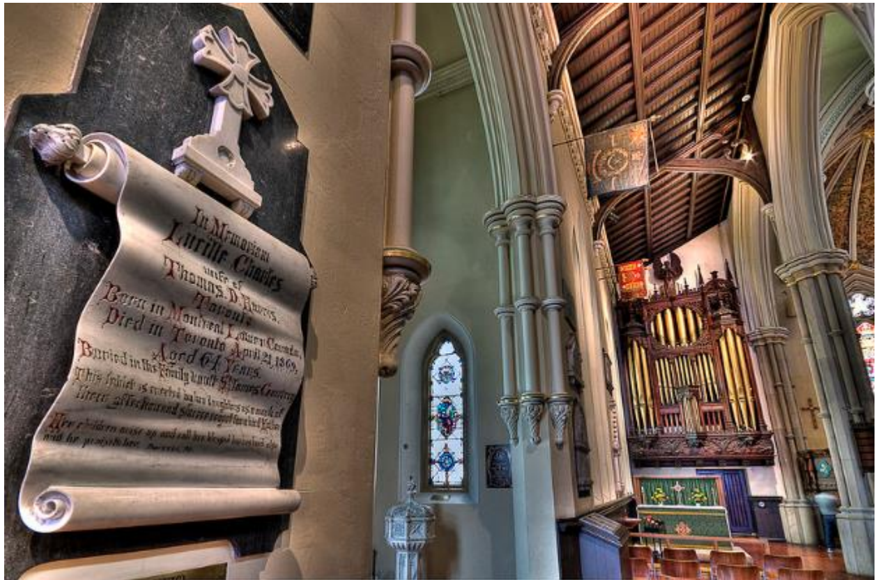
Figure 7 There are eight features in this photo that helps to tame the sound in this church. (1) Marble memorial, (2)the beveled window frames, (3)the pillars,(4) the rounded shapes on the pillars, (5)the pipe organ, (6)the coffered wood ceiling (7) the crown molding to cover the connection from the wall to the wooden ceiling (8) the open wood trusses. It is the sum of all of the parts that makes this room work. St James Anglican Church, Toronto, Ontario, Canada. Photo by Joseph De Buglio
