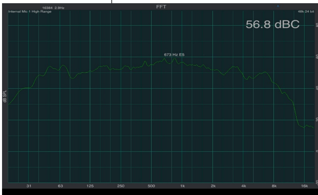
Figure 1 Frequency response with carpeted floors, padded seating, and tube radiator diffusers.
